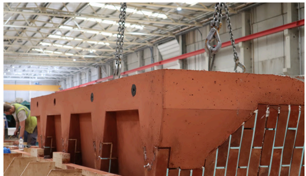
> Panel is lifted out of the mould
