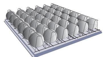
**TYPE 6** In-situ columns with lattice girder slabs and optional spherical void formers
