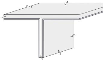
**TYPE 1** Precast twinwall and lattice girder slab with in-situ concrete
