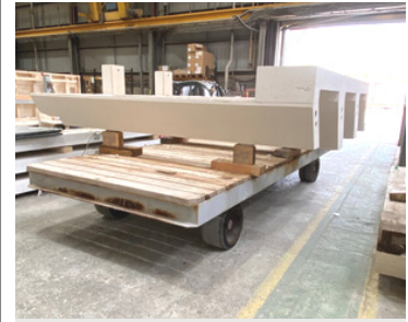
Panel being transported out to the storage yard
