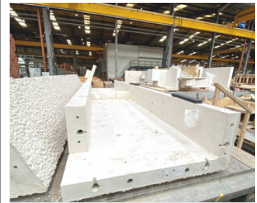
Lifting sockets with slots for temporary drainage
